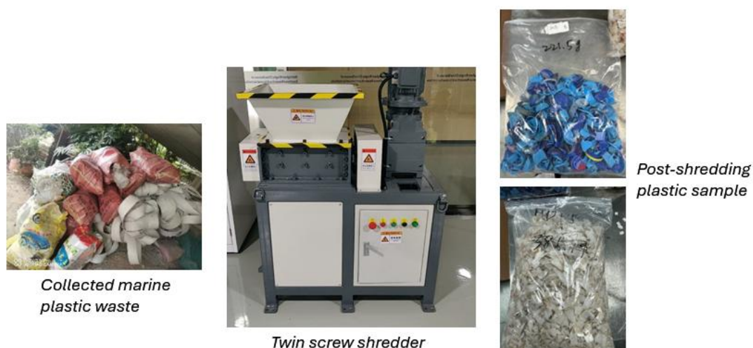
Figure 1. Twin screw shredder for size reduction of collected marine waste plastic
